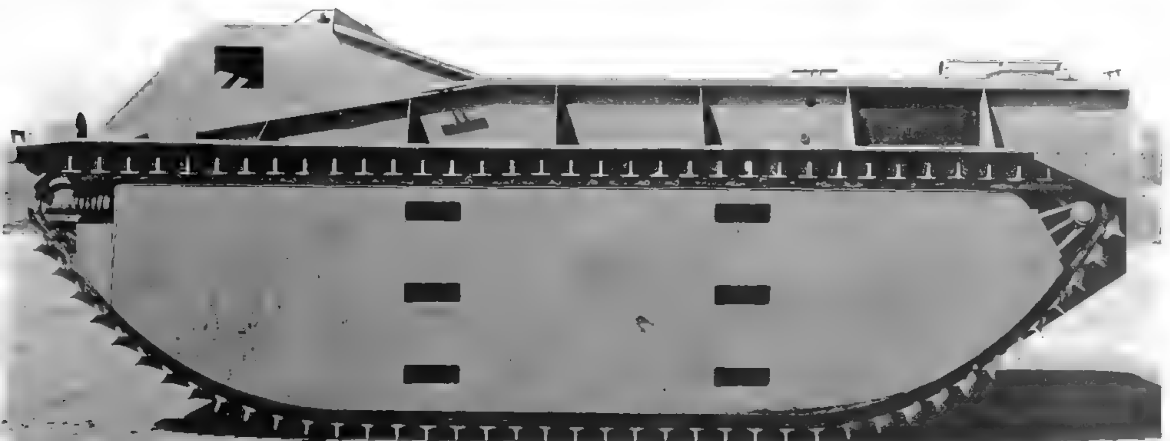
Steps were cut into the sides of the LVT(1) for personnel to use when entering. (National Archives and Records Administration photo)
